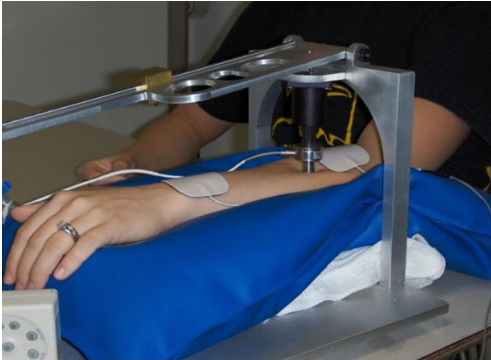
Figure 2-2: Pressure temporal summation measurement during TENS application Pressure device includes a pressure transducer and a lever with a movable weight to grade the force delivered. The pressure stimulus is delivered through a 1 cm 2 probe over the extensor muscle mass.
